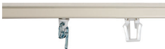
Forest KS Track showing 2 types of wave glider - Eye type on left combined with Steel Zinc Hook inserted & Klick type on right with Forest 2 prong Klick in Hook-klicked into the Wave Glider
